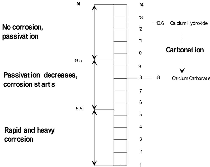
The high alkalinity of cement paste is primarily due to the high calcium hydroxide content (lime) the product of cement hydration as schematically shown in equation 1. Calcium silicate compounds (CS) contained in Portland cement, when mixed with water react and form hydrated calcium silicates (CSH) and Calcium Hydroxide (lime). Lime and other oxides of alkali earth elements, such Sodium (Na) and Potassium (K) create the highly alkaline environment of fresh or "young" concrete.
