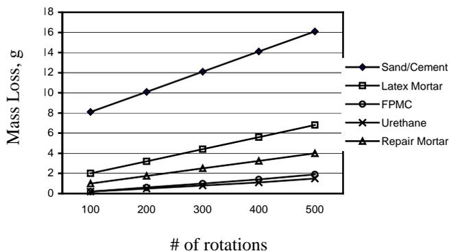
Figure 7. Abrasion resistance of various mortars in wet state – Taber Abrador Model # 503, abrador wheel, Calabrase H-22, mass on each arm =500g.
