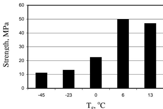
Figure 5. Compressive strength of mortars modified with polymer latexes of varying  $T_g$ . (w/c=0.6, p/c=0.3, sand/cement ratio =2, the control compressive strength of unmodified mortar 41.6 MPa, test temperature 18°C).
